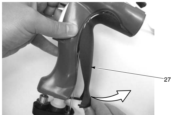
Figure 5-7 Removing the Ground Pad
