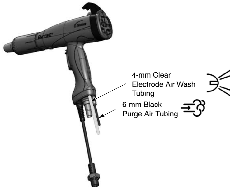
Figure 2-8 Connecting Purge and Air Wash Tubing to the Spray Gun
