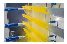
The Encore tube-mount gun is designed for automatic, external and internal cleaning, for use in ultra-fast color-change systems. It is available in two lengths, to accommodate varying powder spray booth widths for coating small to very large products. The gun's width is only 1.93 in. (4.90 cm), minimizing surface area to clean during color change. It also minimizes the width of the booth's automatic gun slot openings, for optimum air flow control.
