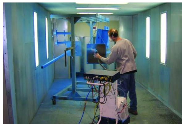
rations. For individual parts or groups of small parts, a compact batch booth might be ideal. Parts are typically hung from a grounded rod in the booth and then manually sprayed with a hopper-fed or box-fed manual electrostatic gun. Compact batch booths are small, economical, and portable. Frequent uses are for cell units, lab units for test panels, or gun cleanout areas.
